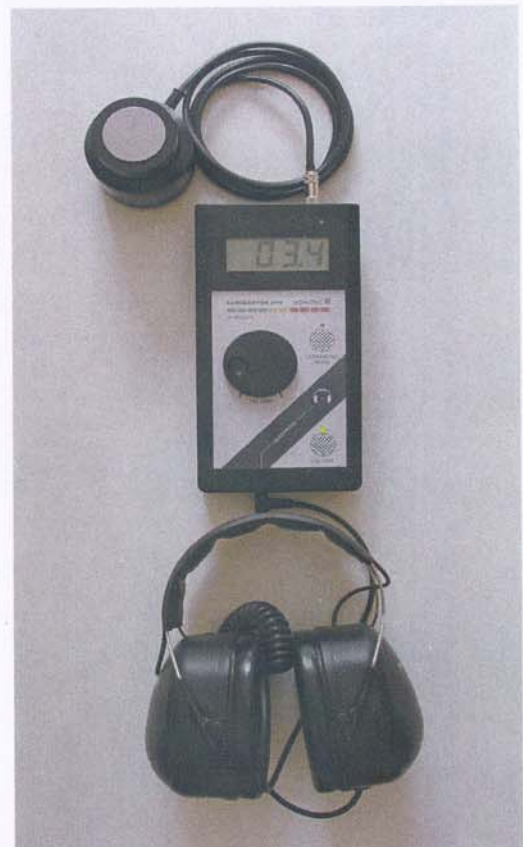
SONAPHONE UH with head phones and ground microphone in the basic set. Possible change-over between acoustic sound and ultrasound
